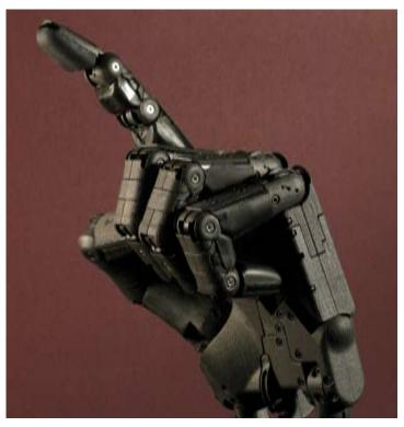
The Shadow Robot Company designs and manufactures state-of-the-art anthropomorphic robot hands and related systems. Graphite produced the parts for one of Shadow's robot hands in their new 'Graphite SLS' material and the company constructed the components incorporating their unique manipulation hardware and sensors.
